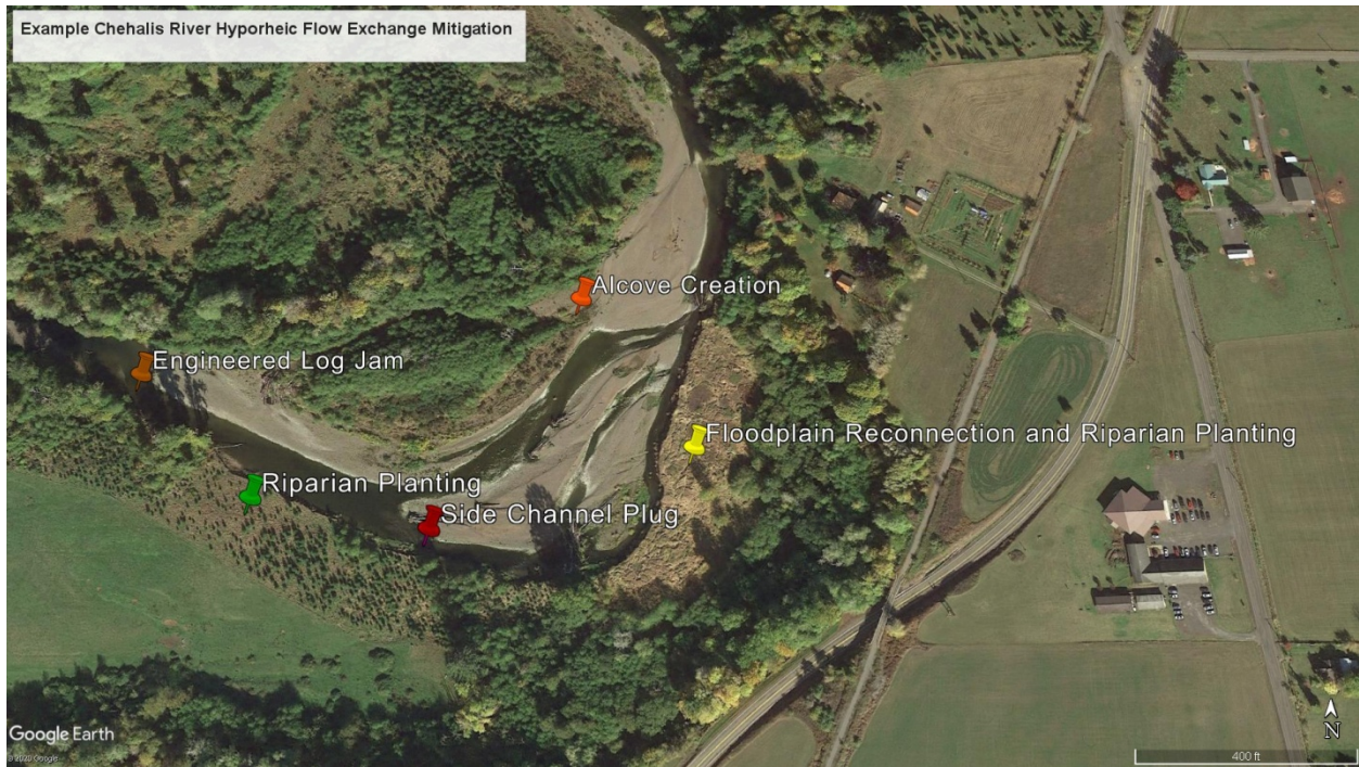
Figure 5: Example Chehalis River Hyporheic Flow Exchange Mitigation Downstream of Pe Ell, Washington.
