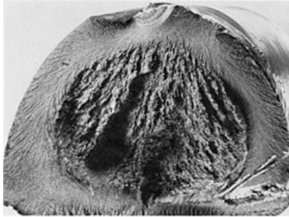
Fig. 2.16 Spiral fracture of a drive shaft of a scooter, starting at surface damage indicated by arrow [20]. a mating halves, b separated halves
