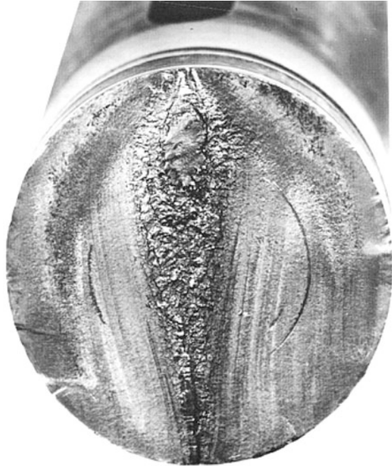
Fig. 2.23 Reversed bending failure in 1046 steel [27]. Rubbing has obliterated the early stages of fatigue cracking. Ratchet marks along circumference indicate locations of crack initiation
