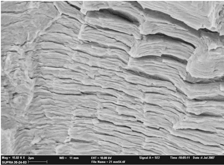
Fig. 2.35 Cracks between striations observed by Milella produced after the crack has passed ductile because the material ahead of crack tip undergoes plastic deformations that produce the typical curved arrays by which they advance on the fracture surface. Brittle striations, instead, develop always on crystallographic planes, usually (100)
