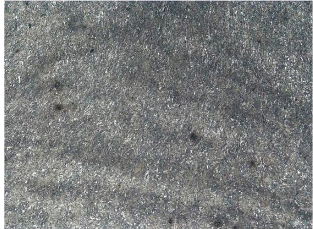
**Fig. 4.** Microstructure of the cross-sectional area of the base plate bolt after etching with 100× magnification.
