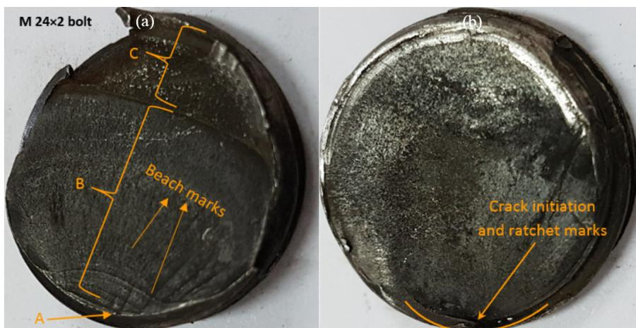
**Fig. 7.** Macro morphology of fracture surface of the radial forging machine bolts threads (zone 2).
