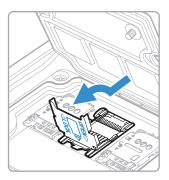
9. Insert the microSD card into the card holder with the contacts facing out.
