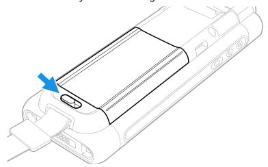
7. Lift up on the edge of the battery and remove it from the computer
