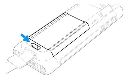
6. Lift up on the edge of the battery and remove it from the computer
