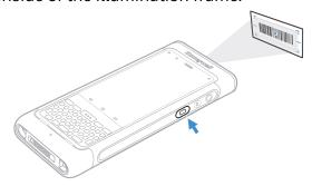
4. Release the Scan button when the computer beeps, and the Scan Status LED briefly turns on. The barcode information is entered into the application in use.
