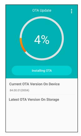
9. Once the installation is complete (100%), select **OK** when prompted to **Reboot** the computer. The computer reboots and finishes the update.
