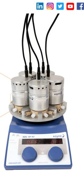
Heating and agitation is provided by any magnetic hotplate stirrer.
