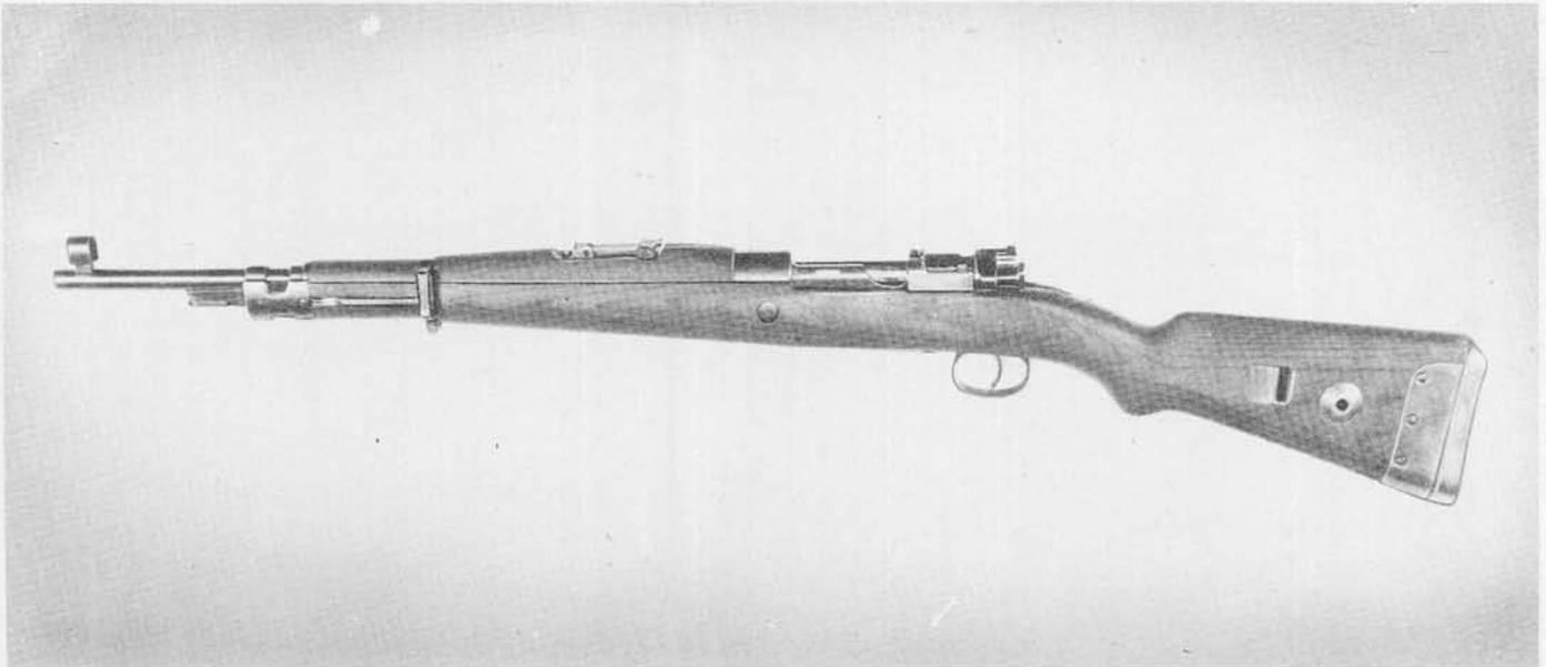
This carbine, a typical Mauser, is very similar to the latest model of the Kar 98K. It is a manually operated, air-cooled, clip-fed shoulder weapon, having a laminated wood stock, a large metal butt plate to protect the stock when grenades are launched, and a sling mounted on the left-hand side.
