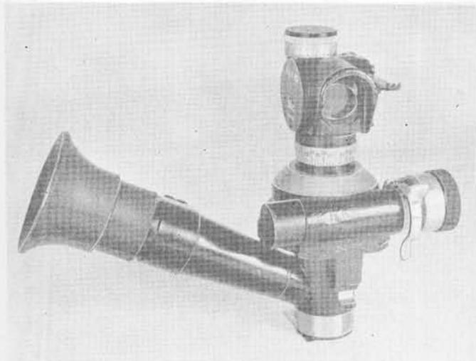
The Rundblickfernrohr 40 is believed to have been designed for use with the 7.5 cm L. G. 40 or the 10.5 cm L. G. 42. A carrying case and two night lighting devices employed with the instrument were also recovered.
