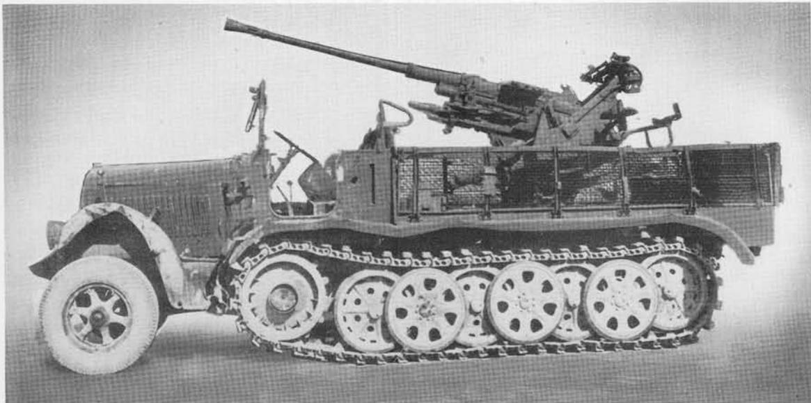
The 3.7 cm Flak 36 has also been mounted on the chassis of the 8-ton medium prime mover described on page 54. Data on the weapon may be found on page 130.1.
