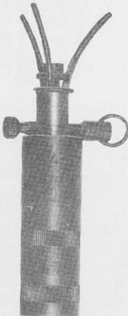
This is the standard igniter used in the "S" mine. It consists of a white metal body, housing the spring-loaded, ball-release type striker assembly. The igniter is provided with a safety pin through the plunger just above the top of the igniter body. There are three pressure prongs attached to the top of the plunger and held in place by a screw. The mine is usually buried with just the prongs of the igniter above the ground.
