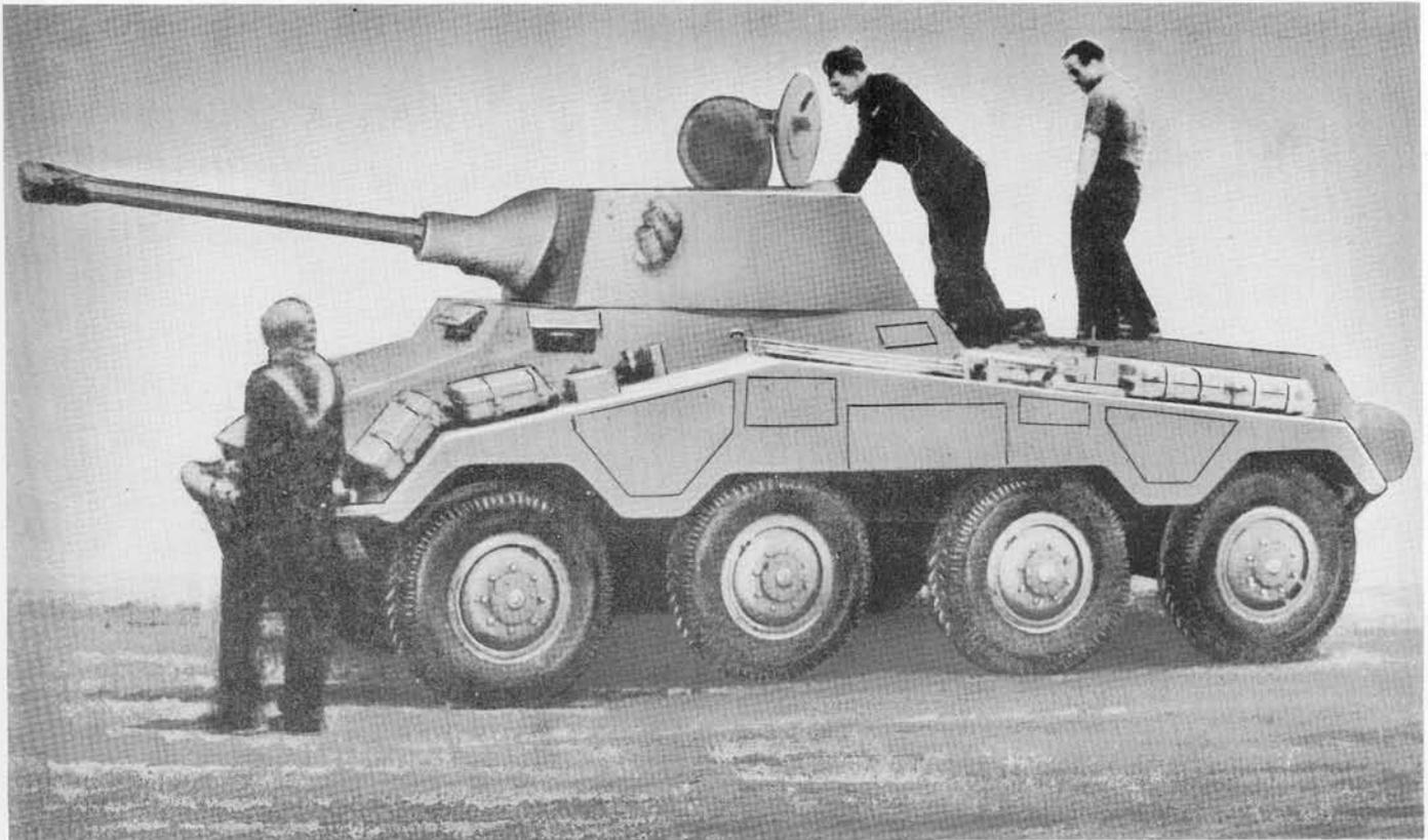
This armored car is basically the 8-wheeled Model Sd. Kfz. 234 equipped with a 12-cylinder, 75°, air-cooled diesel engine. The armor plate on the front of the turret, superstructure, and hull is heavier than that of earlier models. The vehicle, itself, is also about three tons heavier.
