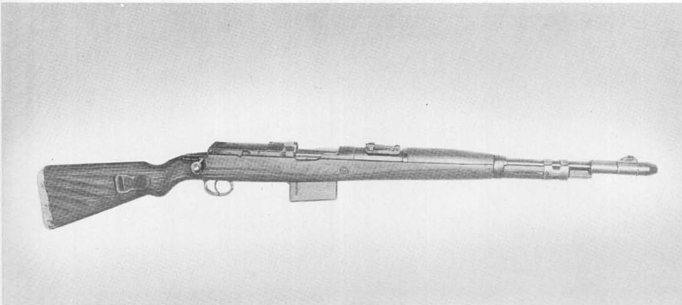
The Gewehr 41 (M) is a self-loading, gas-operated, clip-fed, air-cooled shoulder weapon. It is basically the same as the Gewehr 41 (W) except for several changes that have been made in the manufacture and appearance.
