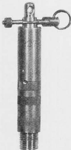
This brass igniter is used with the stock mine and occasionally with the "S" mine. It is also commonly used with booby traps.
