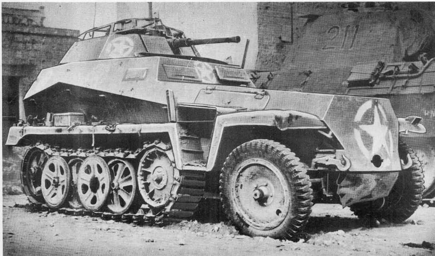
This vehicle, adapted from the light armored personnel carrier, mounts the 2 cm tank gun, Kw. K. 38, and is effective for reconnaissance, action against lightly armored ground targets, protection of troop and supply trains, and as a personnel and supply carrier.
