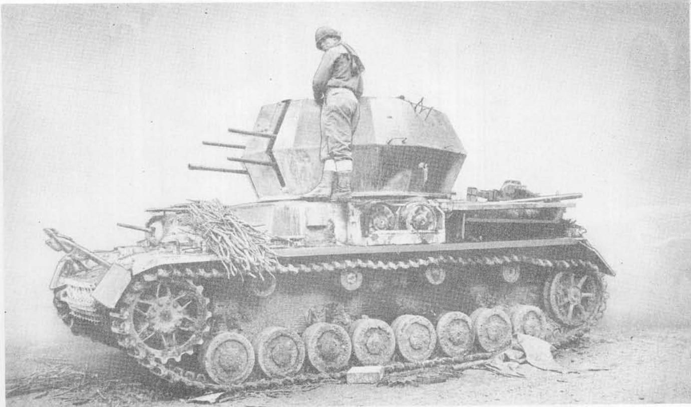
This equipment consists of the four-barrelled 2 cm (.79 in.) anti-aircraft gun mounted on the Pz. Kpfw. IV chassis. The gun has been mounted in an open topped, nine-sided turret. Elevation is from 10° to 90° and traverse is 360°.
