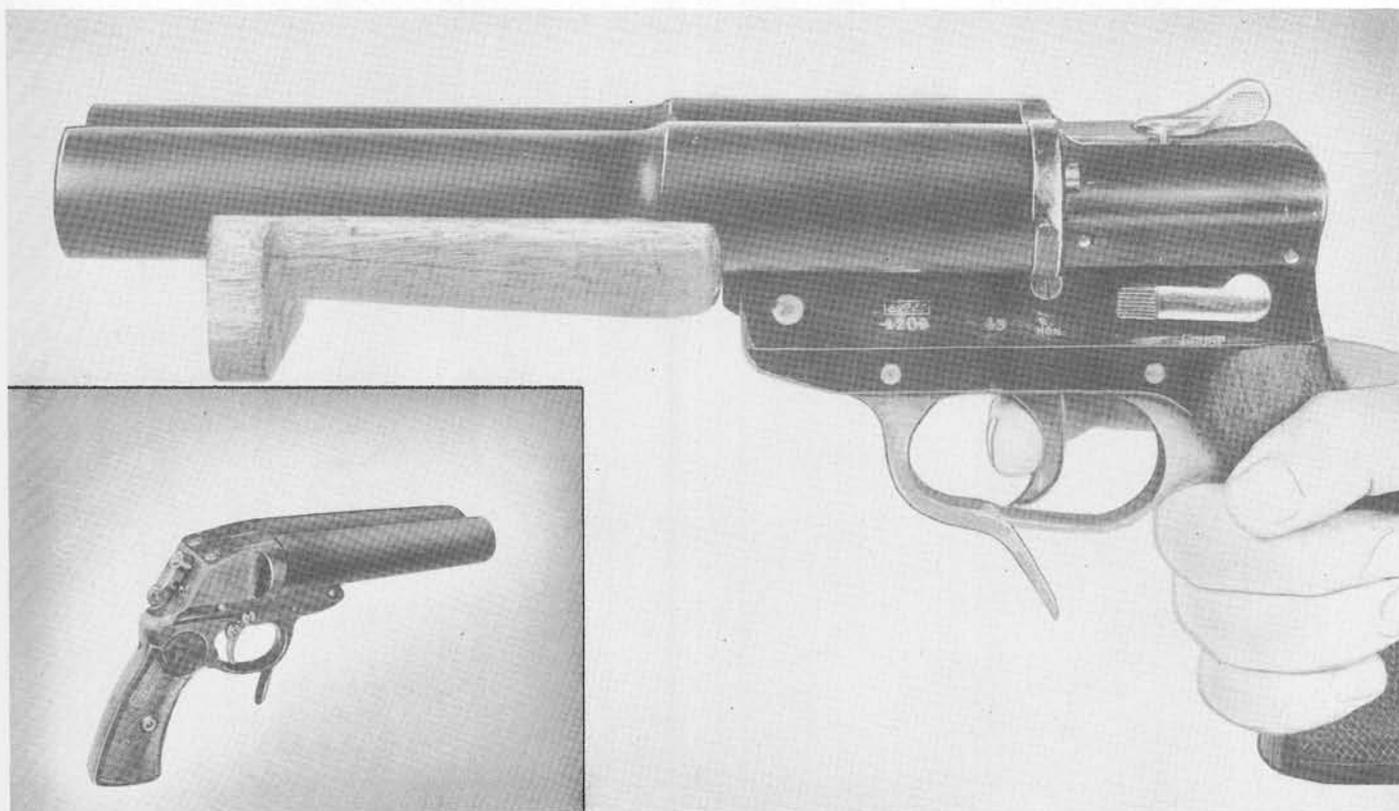
The 27 mm double barrel signal pistol is unique in that the basic parts such as the trigger, trigger-guard, lever release, hammer assembly and switch lever, as well as all pins, are made of steel; the remaining parts, with the exception of the wooden fore-stock and hand grips, are made of an aluminum alloy.
