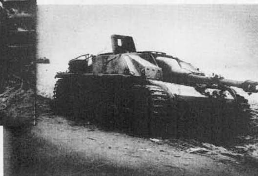
This equipment, consisting of the 7.5 cm Stu. K. 40 (L/48) mounted on the Pz. Kpfw. IV chassis, represents a further development in German assault guns. The design follows that of its predecessor, the Stu. G. 40, mounted on the Pz. Kpfw. III chassis, with the exception that in the later equipment the usual keystone gun mantlet has been replaced by a cast steel mantlet with curved surfaces to offer the maximum projectile deflection. The mantlet, 130 mm thick, houses the buffer and recuperator.
