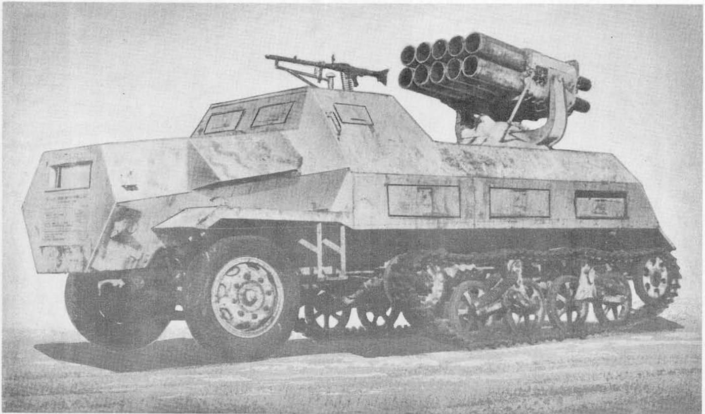
The chassis of this self-propelled rocket projector follows the half-track design but differs materially from the standard German half-track series of prime movers.
