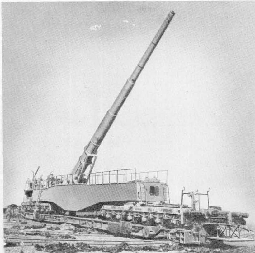
The German 28 cm K5 (E) has an unconfirmed range of 31 miles and fires a pre-engraved projectile weighing approximately 550 pounds. It is fired from a turntable affording a 360° traverse.
