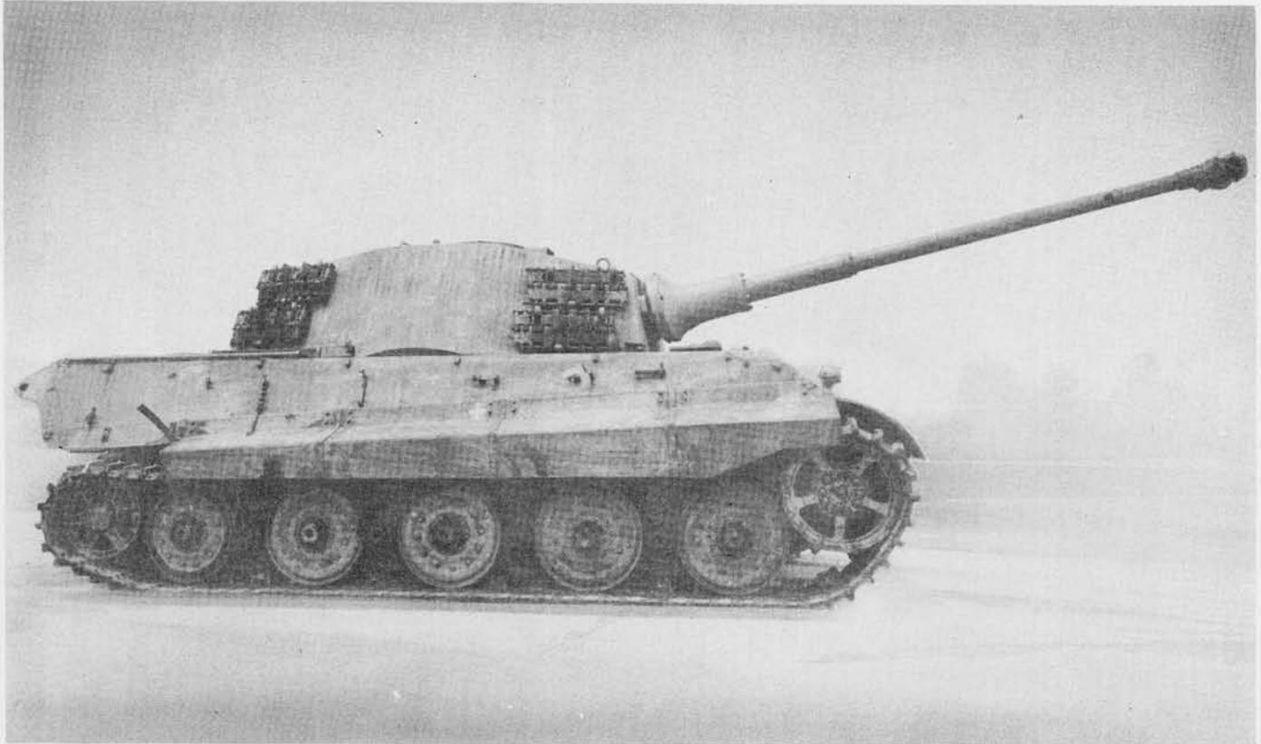
This heavy tank designed for defensive warfare or for penetrating strong lines of defense made its combat appearance in 1944. It is distinguished by heavy frontal armor and by the employment of the heaviest German gun to be used in a turret with 360° traverse—the 8.8 cm Kw. K. 43 (L/71). This gun has a muzzle velocity of 3,280 f/s, and firing an A.P.C.B.C. projectile weighing 22.4 pounds against 30° homogenous plate has a reported penetration of 6.3 inches at 1,000 yards.
