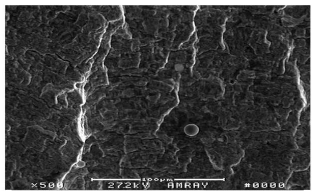
Figure 18 A 500X SEM photo of the area just above the origin shown in Figure 17 reveals fatigue fracture features
