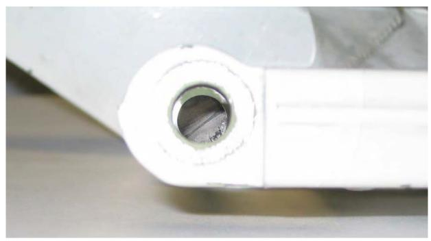
Figure 4 This photo is looking through the drag link assembly hole that reveals a dark narrow band running diagonally through the center of the bolt fracture surface from 8 o'clock to 2 o'clock. There is a semi-circle at the 11 o'clock position and rough edge at the four o'clock
