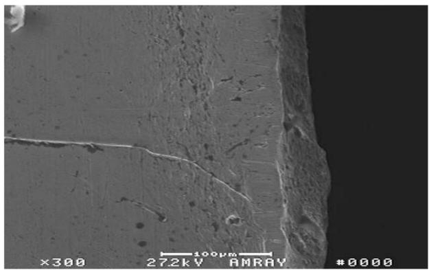
Figure 22 A 300X SEM photo of the outlined area in Figure 21 shows the wear.
