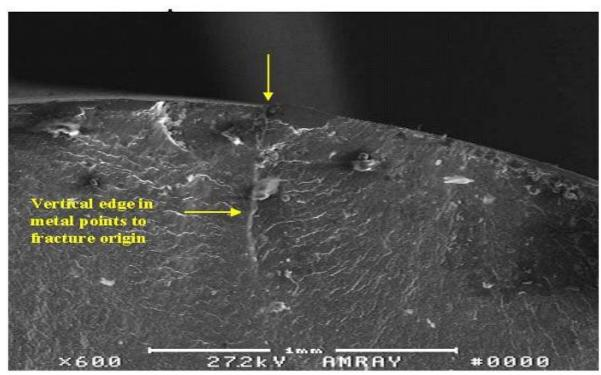
Figure 11 A 60X SEM photo showing the semi-circular shaped area at the bolt's top edge in figure 5. The origin is at the outer surface and indicated by the arrow. Note the vertical feature in the metal that also points to this edge
