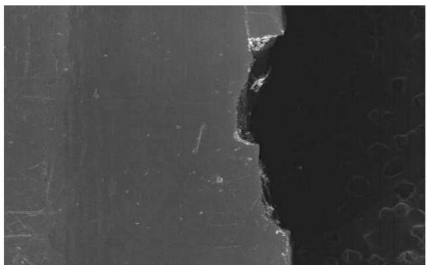
Figure 19 A 30X SEM photo of the side of the bolt at the 6 o'clock area from Figure 5 shows some wear and a crack
