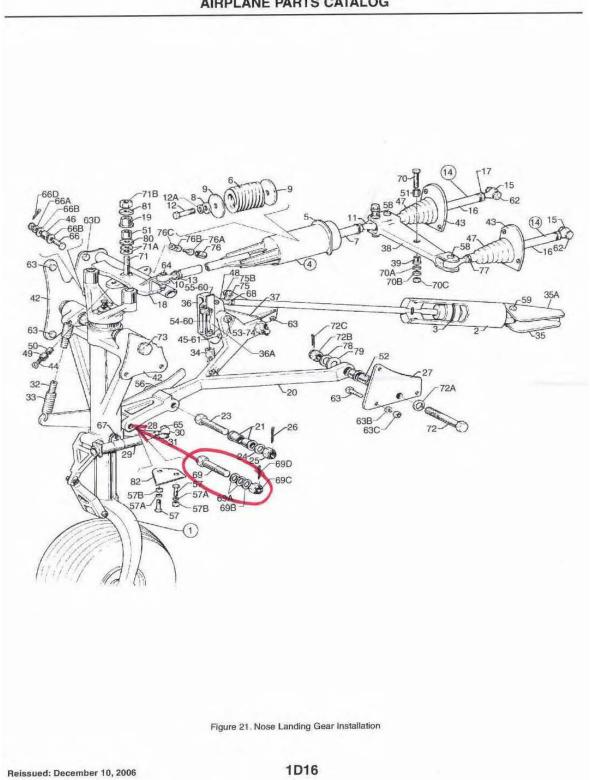
Figure 1 Figure item #69 is the bolt that failed. It is PN 400-191, an AN5-51 bolt.
