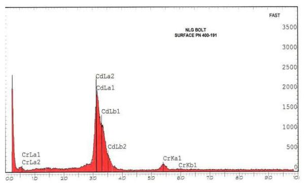
Figure 25 The bolt outer surface is plated with cadmium and a chromate conversion coating.
