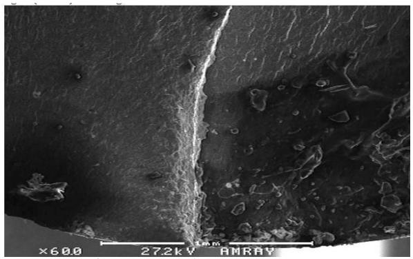
Figure 17 A 60X SEM photo of the bottom origin at the 6 o'clock position as shown in Figure 16.
