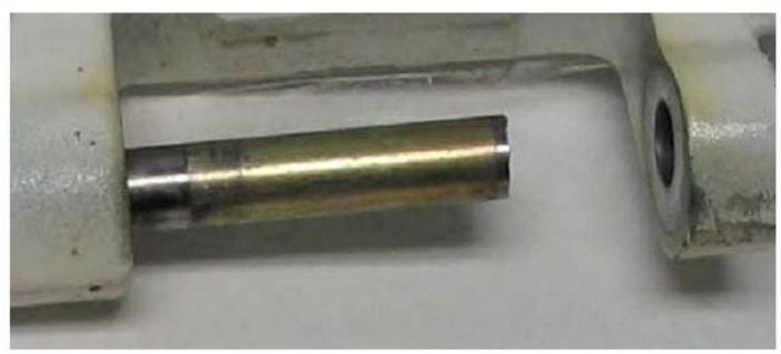
Figure 23 The gold color is removed from the bolt very near the fracture zone.
