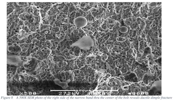
Figure 8 A 500X SEM photo of the right side of the narrow band thru the center of the bolt reveals ductile dimple fracture features characteristic of instantaneous final fracture.
