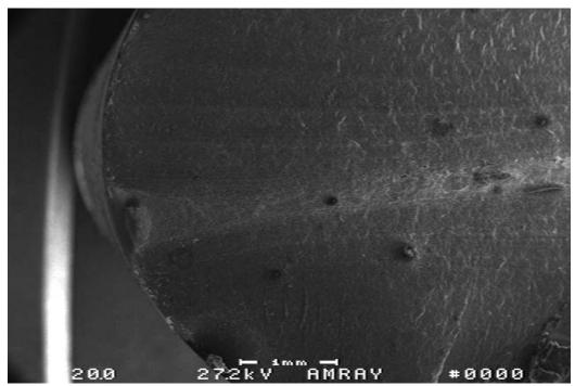
Figure 7 A 20X SEM photo of the left side of the narrow center band. The description of the beach marks discussed in Figure 6 also applies here
