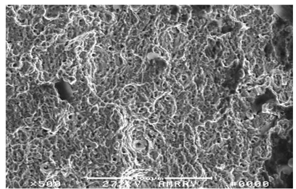
Figure 9 A 500X SEM photo of the center section of the narrow band reveals similar fracture features characteristic of overload.
