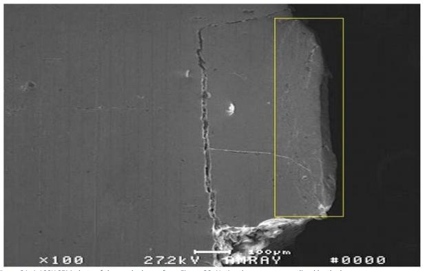
Figure 21 A 100X SEM photo of the cracked area from Figure 20. Notice the wear area outlined by the box
