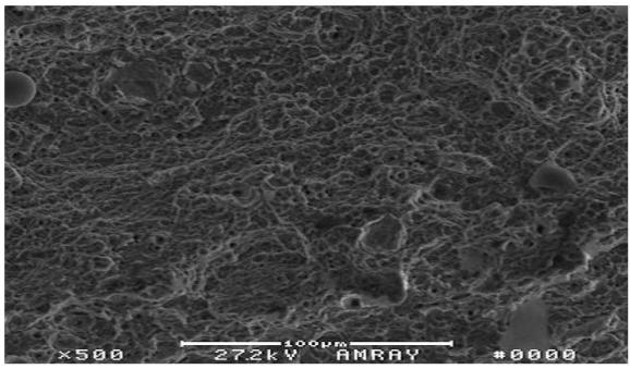
Figure 10 A 500X SEM photo of the left side of the narrow band in the center of the bolt also reveals the ductile dimple fracture features characteristic of instantaneous overload.
