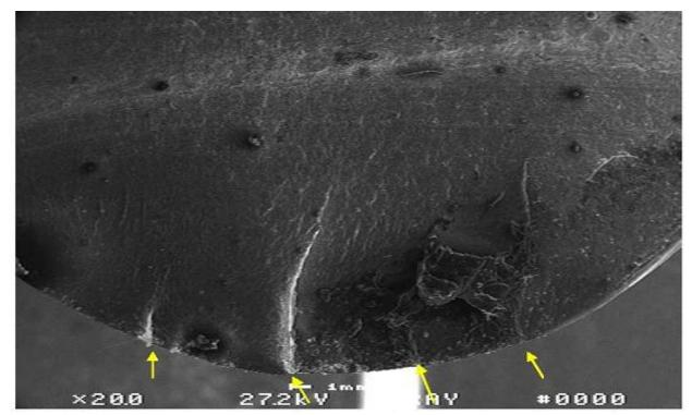
Figure 16 A 20X SEM photo of the bottom edge of the bolt from Figure 5 shows multiple origins (arrows) at the edge
