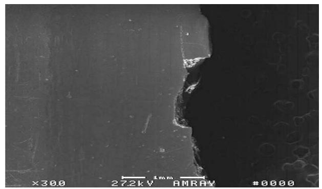
Figure 20 A 30X SEM photo of the side at the 6 o'clock fracture origin shows a crack on the surface.
