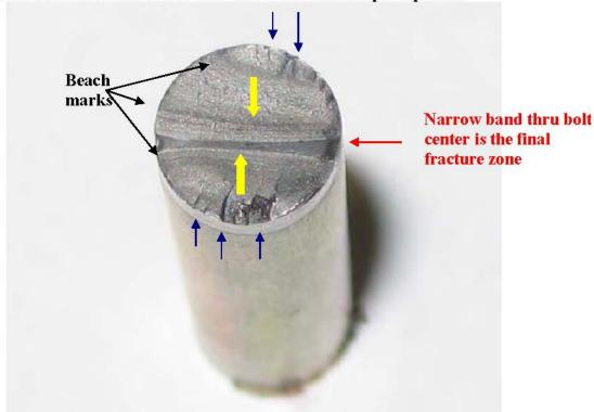
Figure 5 This photo shows the bolt fracture surface with appropriate areas labeled. Blue arrows are fracture origins. Large yellow arrows indicate crack growth direction by fatigue.
