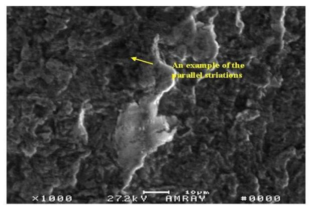
Figure 14 A 1000X SEM photo of an area just below the top origin shows parallel striations characteristic of fatigue crack growth
