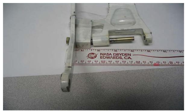
Figure 2 This photo shows the bolt still stuck in the drag link assembly, Figure item 20 in Figure 1.
