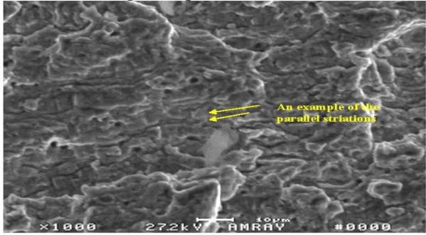
Figure 15 A 1000X SEM photo of an area below the top origin and above the final fracture at the center of the bolt shows parallel striations characteristic of fatigue crack growth. Crack growth direction runs from top to bottom.
