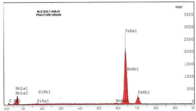
Figure 24 The base metal of the bolt is low alloy carbon steel.
