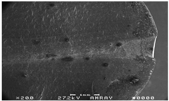
Figure 6 A 20X SEM photo of the right side of the narrow dark band running through the center of the bolt. Notice that the beach marks above the center band are concaved upwards, and those below the center band are concaved downwards.
