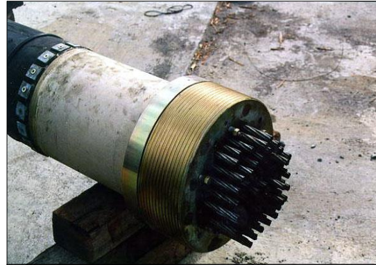
Wire strands within stay cables
